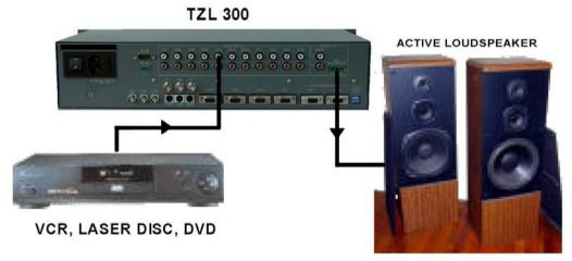
The balanced and unbalanced outputs level can be modified using the IR remote control or via RS232/RS485.
