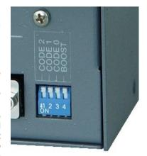
RS232 standard and the connection is of the point-to-point type. In this case, the address must be OFF, OFF, OFF as per factory setting.
